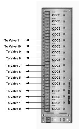
Figure IV-7. MAIDEN Solid-State Relay Board
