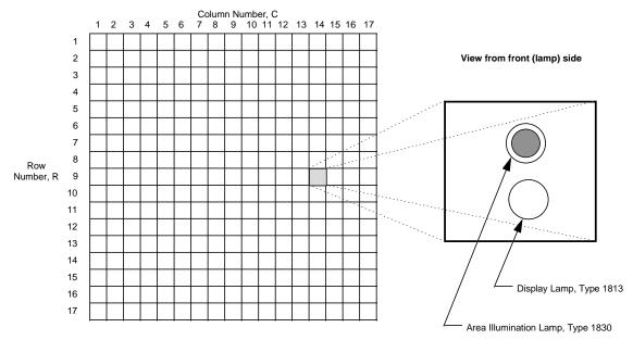
Display lamps are individually addressable. The row driver completes the ground circuit for all lamps in a specified row. The column driver supplies power to all lamps in a specified column.
