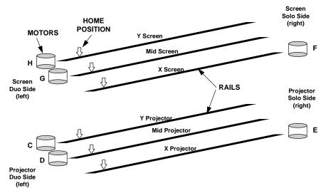
Figure III-1. Screen/Projector Schematic
