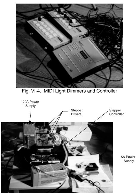
Fig. VI-5. Stepper Motor Drivers and Controller
