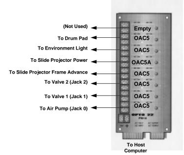
Figure II-5. Solid-State Relay Board
