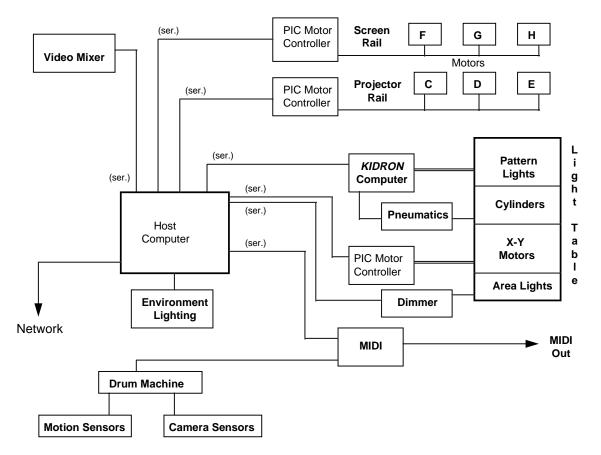
Figure III-6. The RAILS System
