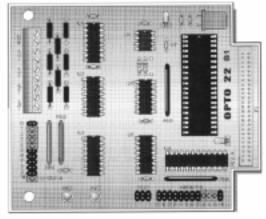
Figure IV-6. Opto22 Brainboard, Model B1
