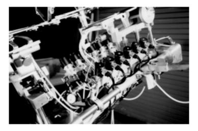
Figure IV-2. Pneumatic Solenoid Valves
