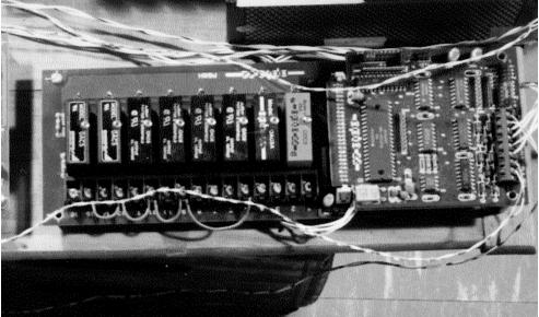
Figure V-4. SCRIBE Relay Board and Brainboard
