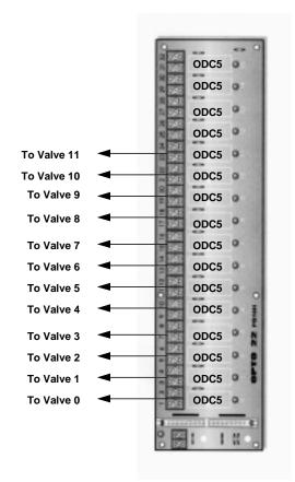
Figure IV-7. MAIDEN Solid-State Relay Board
