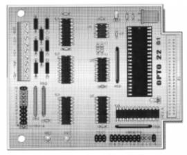
Figure IV-6. Opto22 Brainboard, Model B1
