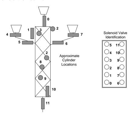
Figure IV-3. Cylinder-Valve Correspondences
