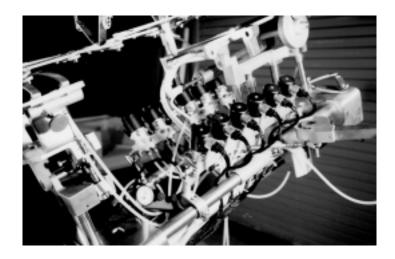
Figure IV-2. Pneumatic Solenoid Valves
