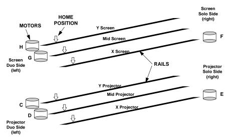
Figure III-1. Screen/Projector Schematic
