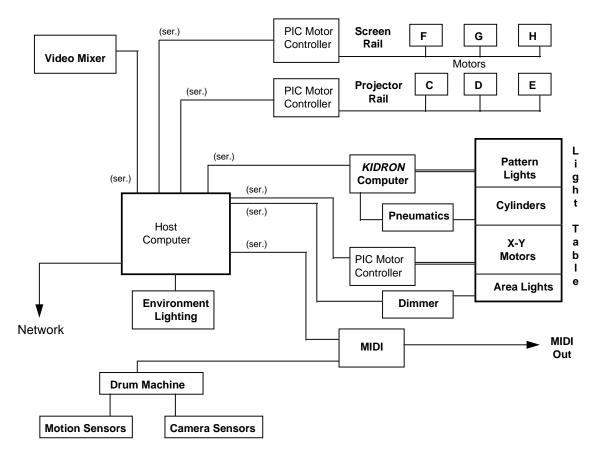
Figure III-6. The RAILS System
